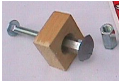
Carriage bolt, wood block, and coupling nut.
