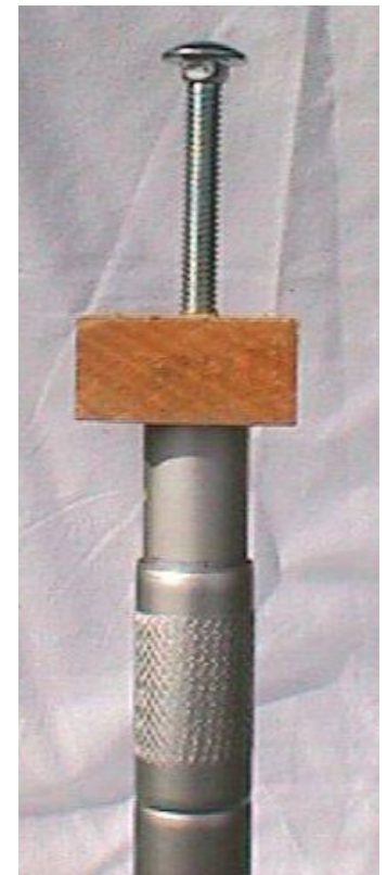
Centering block in position to hold the coupling nut while epoxy sets.
